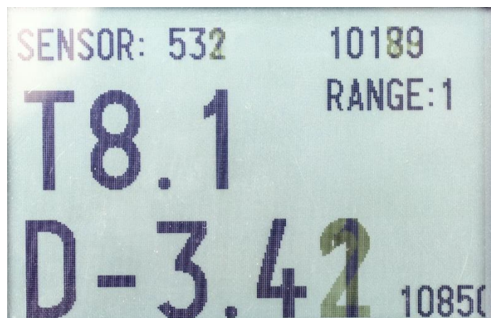
Figure 22 - Aperture test showing a 3.41 stop difference between T2.5 and T8.1
