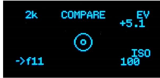
Comparing the averaged EV to various points in the scene (EV readout changes from absolute to relative)
